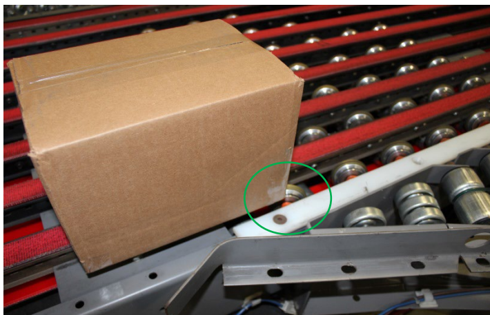
Correct alignment – product contacts the first spur side divert wheels.
