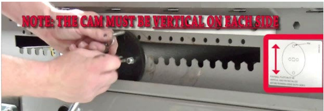
The Cams must be vertical on each side.
